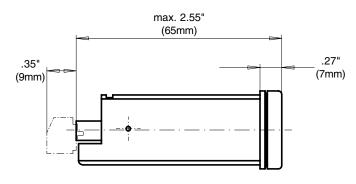
Maximum panel mounting thickness: 0.4" (10mm)
